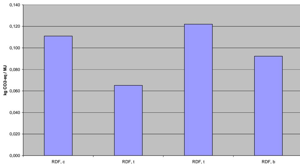
RDF used as fuel in cement ovens also performs well. The alternative where digestion is combined with mechanical separation is the best one.
