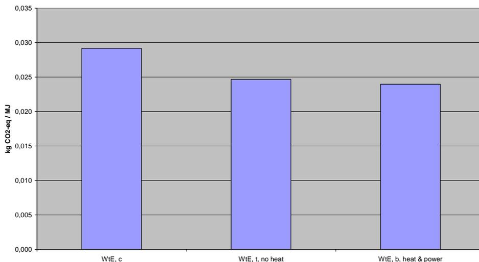
Due to the allocation of part of GHG emissions to the waste treatment service, the performance of the WtE chains is good.
