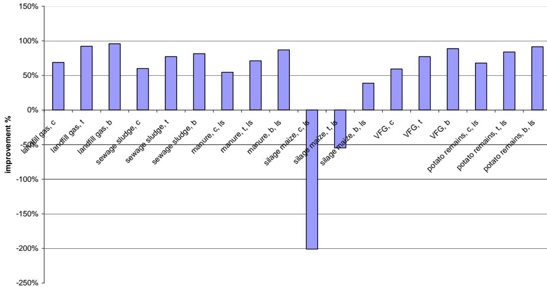
Improvement percentages for WtE chains and digestion chains are high, from 85 to 97%. Landfill gas improvement percentages are a little higher for use in CHP to make electricity than for use as green gas for heating. This is due to the different fossil references for both systems: electricity from grid vs natural gas for heating.
