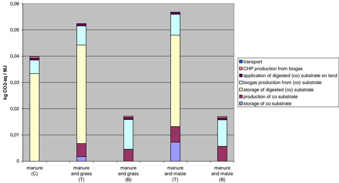
Storage is the important source of emissions. In the best practice chains, storage emissions are assumed to be zero: this improves performance significantly. Crop cultivation is also important, especially in best practice chains where leaks are closed in the storage system.
