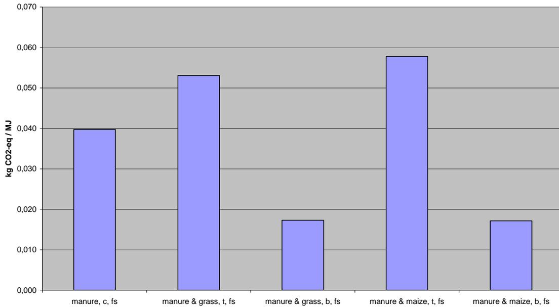
Looking at the digestion chains, co-digestion unexpectedly leads to worse results. This is due to the fact that manure is considered a waste, but the co-digested crops are products. For manure, the previous chain is cut-off, while for maize and grass their production chains are included according to the allocation rules. Best practice chains indeed have least GHG emissions.
